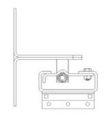
JAMBS MUST BE SQUARE AND PLUMB A MINIMUM OF 3-1/2 INCH WIDE JAMBS REQUIRED TO MOUNT HARDWARE
