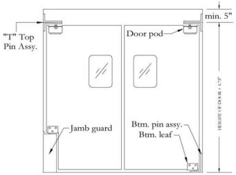
NOTE: Bottom pin assembly must be secured to floor.
