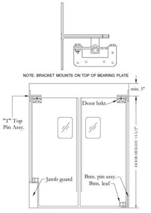
NOTE: Bottom pin assembly must be secured to floor.
