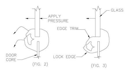
3. FOR EASE IN REPLACING NEW WINDOW, LUBRICATE RUBBER MOLDING WITH A LIQUID WINDOW CLEANER. SPREAD THE MOLDING AND START GLASS INTO POSITION (FIG. 4). FORCE ACRYLIC TO TOP OF MOLDING. USE TOOL AT BOTTOM BETWEEN GLASS & RUBBER. APPLY PRESSURE UNTIL GLASS SEATS IN POSITION.
