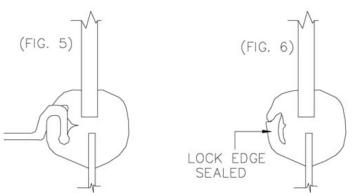
4. TO SECURE GLASS IN MOLDING START HOOKED END OF TOOL UNDER LOCKING EDGE OF RUBBER (FIG. 5). WITH SLIGHT PRESSURE AND SLIDING MOTION WORK TOOL AROUND ENTIRE WINDOW OPENING. (FIG. 6) SHOWS LOCK EDGE CLOSED.
