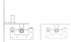
NOTE: BRACKET MOUNTS ON TOP OF BEARING PLATE
