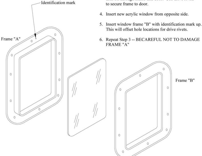
NOTE: For through bolt installation, must have one of the identification marks DOWN to align holes.
