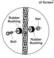
Affix the Rubber Bushing Chain Stopper through the marked link like the illustration above.
