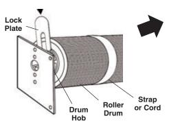
First, wind up the screen so it is completely on the Roller Drum. Using a strap or cord, secure the screen so it is unable to unwind. Place the Lock Plate into the Drum Hub.
