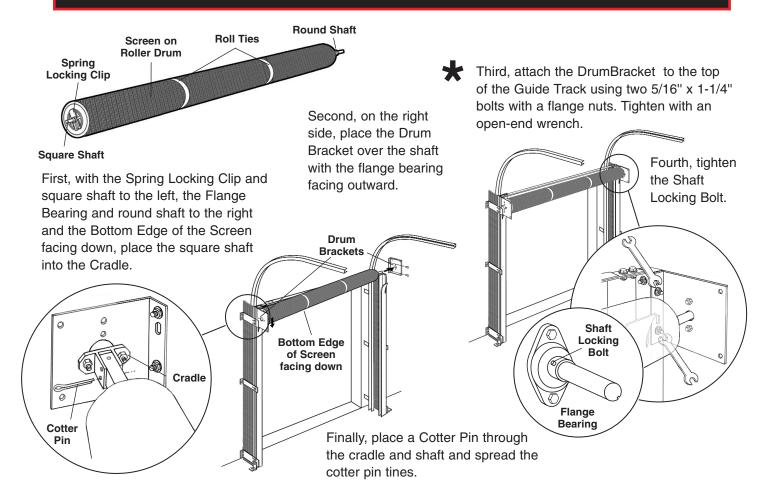
At this point the Screen Roller Drum must be leveled. The Drum Bracket Mounting Bolts on one or both sides can be loosened and the drumcan be accurately leveled.
