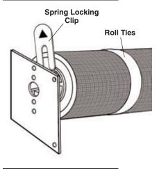
With the Screen Roller Drum in place, remove the Spring Locking Clip.
