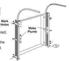
Remove assembly and drill all 10 holes. If you are mounting to a concrete wall or concrete block, wall, anchors will be necessary (not supplied).
