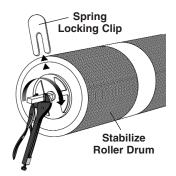
Finally, with the Roller Drum totally stabilized, lock a Vise Grip onto the shaft. Keeping everything in tension, remove the Lock Plate. Turn the shaft clockwise one complete turn and replace the Spring Locking Clip.
