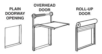
There are a variety of doors used at both industrial and commercial facilities. Each has its specific opening/closing mechanism. This Screen-Pro unit has been shipped with hardware to accommodate a Stand-Off Mounting Method. It should be mounted in front of any rails or guide tracks and centered on the doorway opening. Also, the Screen-Pro guide tracks should be on the outside of any rails or tracks used with the security (regular) door.
