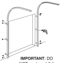
NOT mark or drill the Floor Anchor Bracket mounting holes. That is Step 13, Page 7.
