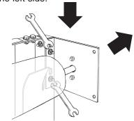
Next, detach the right side Drum Bracket from the right Guide Track. Then lift the Screen Roller Drum out of the left Drum Bracket cradle.
