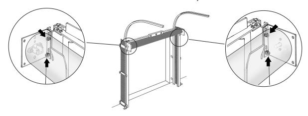
of the Hoist Pulley Assembly through the 2 Chain Guides.
