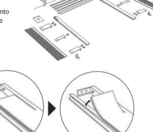
Using work horses will make the assembly process easier although it is not essential. Place the Guide Tracks on the horses with the Guide Flare Plate facing up.
