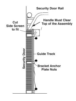
**TIP**: It is much easier to do this procedure when the security door is open.
