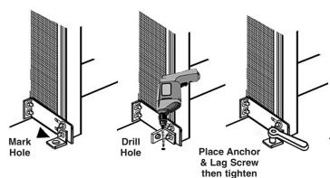
Next, the Screen-Pro should be fastened to the floor using the Floor Anchor Angles which were attached to the Bottom Track Braces (left & right) in Step 6. First, mark the holes. Second, drill the holes. Finally, place the screw anchors and secure with a lag screws.
