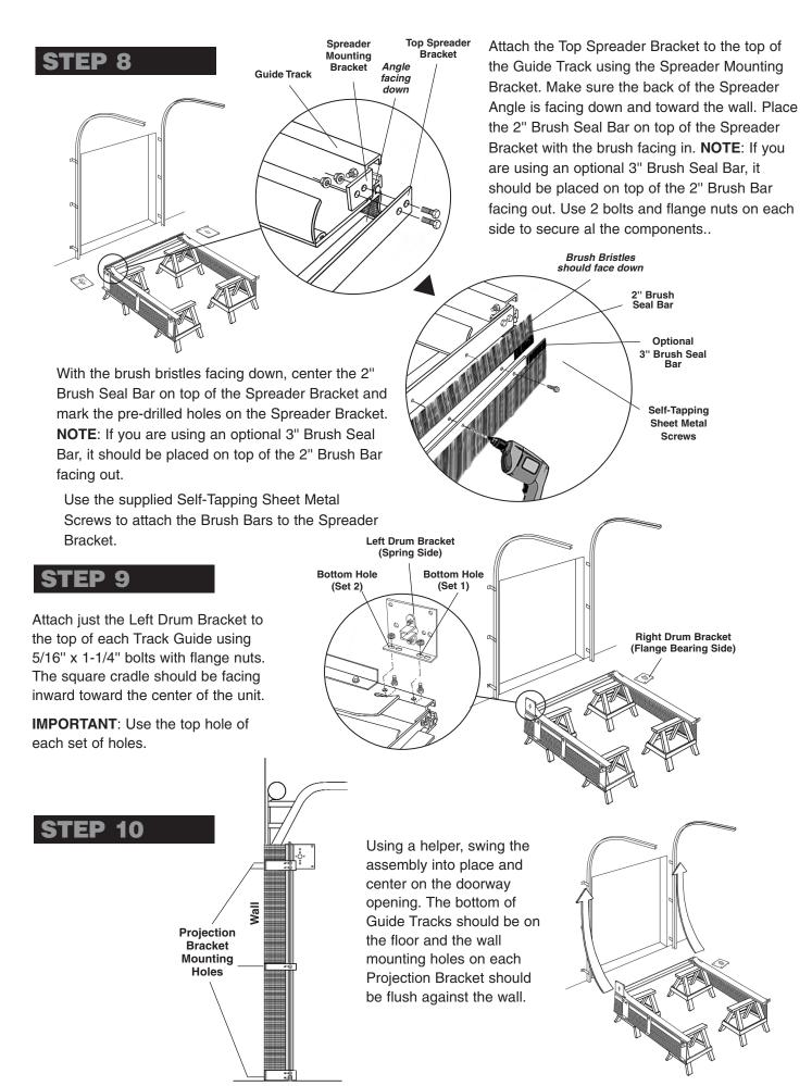
Once the assembly is centered, make sure that each Guide Track is plumb. Then mark the Projection Bracket mounting holes.
