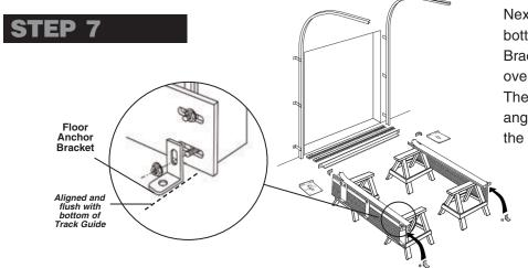
Projection Bracket is perpendicular to the Guide Track. Then tighten with a wrench.
