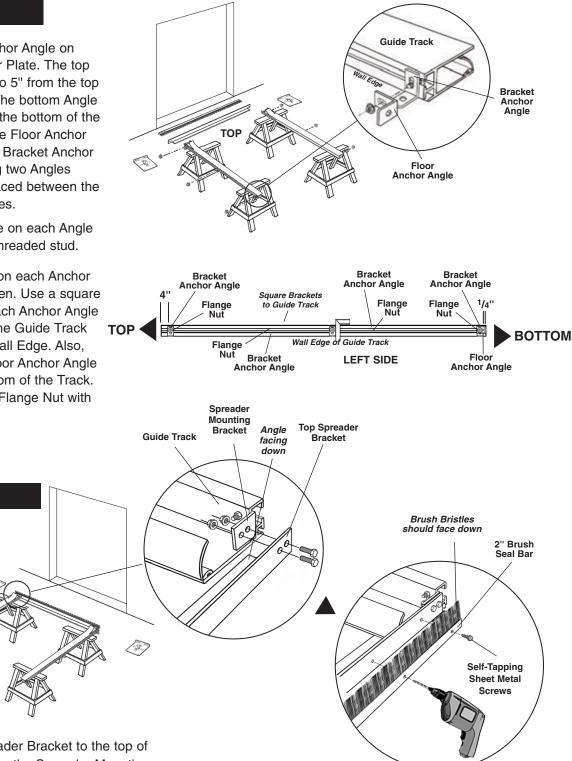
Attach the Top Spreader Bracket to the top of the Guide Track using the Spreader Mounting Bracket. Make sure the back of the Spreader Angle is facing down and toward the wall.
