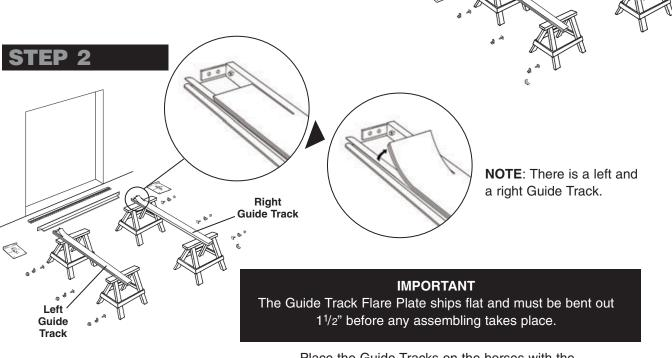
Place the Guide Tracks on the horses with the Guide Flare Plate facing up.
