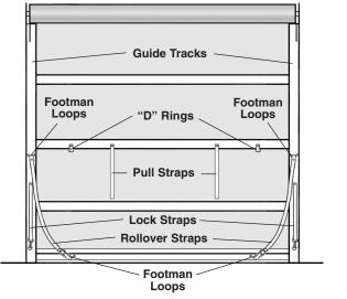
Feed the strap through the Footman Loop that has been pre-attached to the Guide Track. Then take the strap back through the slide as shown in the illustration to the right. Adjust the strap so it is taut when the door is in the open position.
