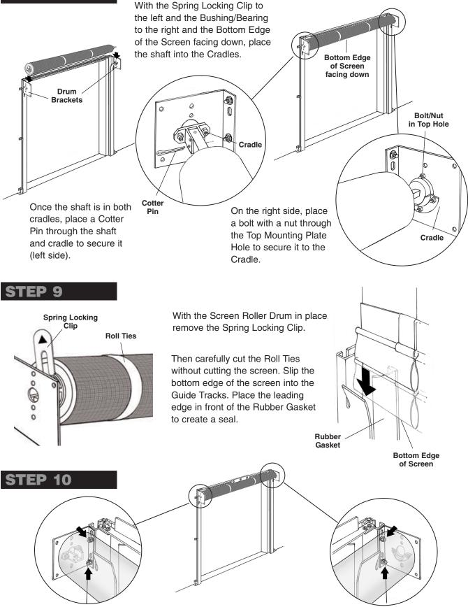
At this point the Screen Roller Drum must be leveled. The Drum Bracket Mounting Bolts on one or both sides can be loosened and the drum can be accurately leveled.
