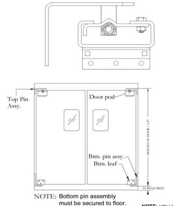
JAMBS MUST BE SQUARE AND PLUMB A MINIMUM OF 3-1/2 INCH WIDE JAMBS REQUIRED TO MOUNT HARDWARE
