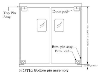
must be secured to floor.
